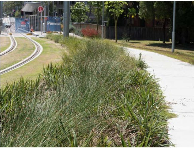
Figure 27. Low planting can be used to separate pedestrian paths from non-pedestrian zones (PLR, Ngara)
