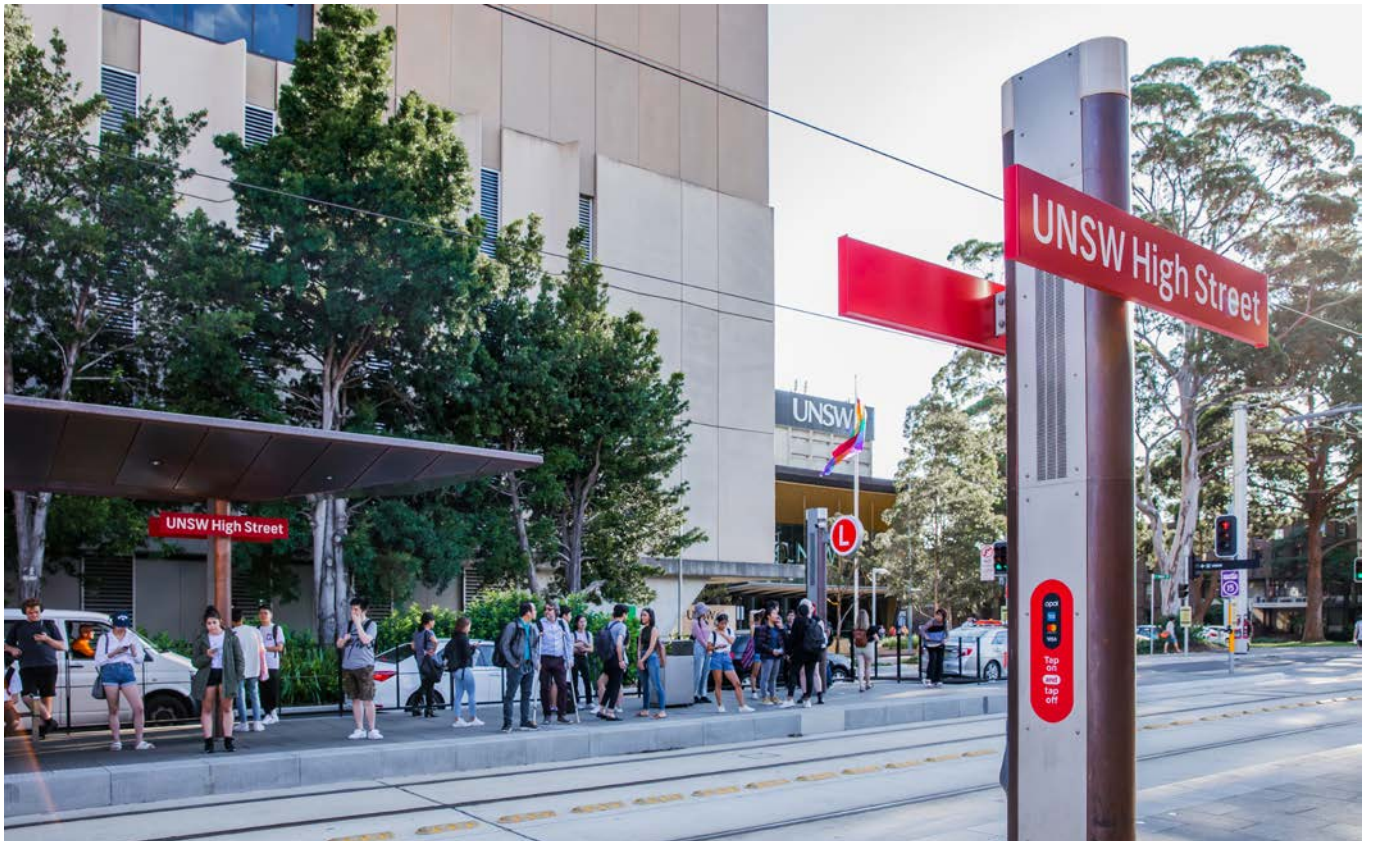
Figure 149. Clutter free platforms maximise space for customers (CSELR, UNSW High Street)
