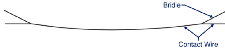
Figure 6 – Typical span configuration for trolley wire system
