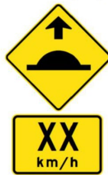
Figure 5 – Warning signs in advance of the RSP
