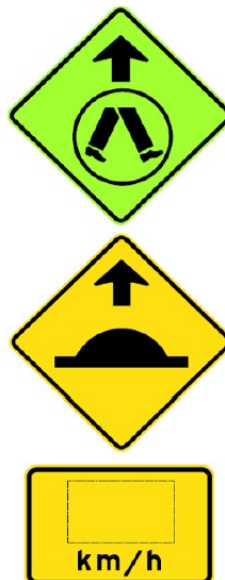
Figure 7 – Warning signs in advance of an RSP, when a pedestrian crossing is incorporated with the RSP
