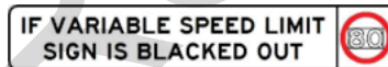
Figure 18 – If variable speed limit sign is blacked out – tunnel use only' sign (G6-317-1N)
