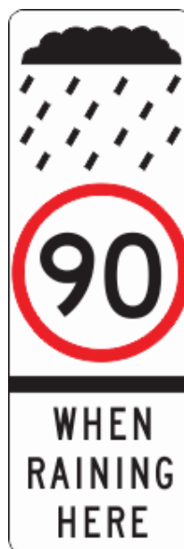
Figure 23 – 'Speed restriction – when raining here' sign (R4-238N)
