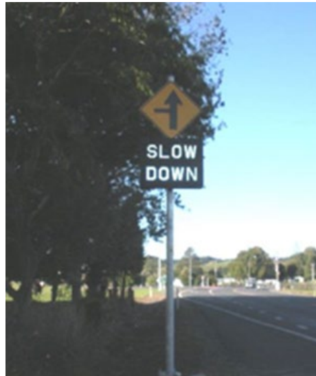
Figure 6 – Example 1 of alternative forms of RISZ that should not be used in NSW (Source: Mackie et al., 2014, New Zealand's Rural Intersection Active Warning System ) and Bradshaw et al., 2013)
