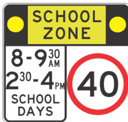
Figure 47 – Flashing school zone sign
