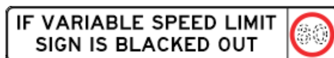
Figure 25 – If variable speed limit sign is blacked out sign (tunnel use only) (G6-317-1N)
