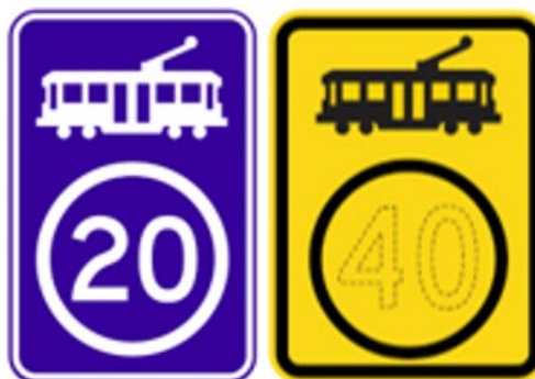
Figure 16 – Advisory tram speed limit sign (G9-N390n + W1-10)
