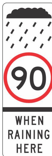
Figure 29 – Speed restriction when raining here sign (R4-238N)
