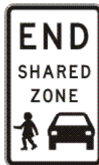
Figure 41 – End shared zone sign (R4-5)
