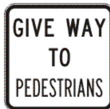
Figure 40 – Give way to pedestrians sign (R4-10)
